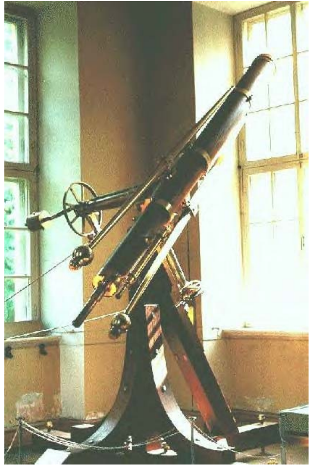
Figure 3: The Fraunhofer 9-inch "great refractor" used by Struve at the Tartu Observatory in Dorpat, Estonia.
