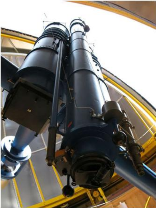
Figure 5: Photo of the Bruce astrograph made by the author in 2009, left astrograph with plate B, right telescope is for tracking control, behind it is the second astrograph with plate A
