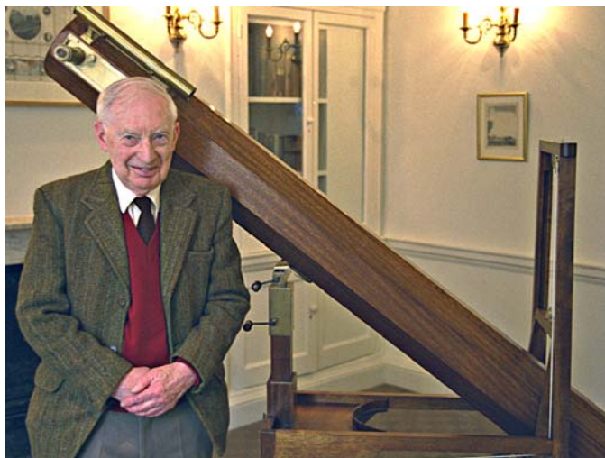
Figure 2: Shown above is the type of telescope that Herschel probably used for his double star measurements. If you look at the telescope stand carefully, you'll see two small keys that the observer turns to follow the sky in altitude and azimuth. It probably wasn't a bad system. Herschel made over 200 telescopes with apertures between 6 and 9 inches on alt-azimuth stands similar to the one shown above. He sold them to support himself. The photograph above was taken by Richard Berry of his friend Brian Manning, a very accomplished amateur astronomer, at the Herschel Museum in Bath, England.
