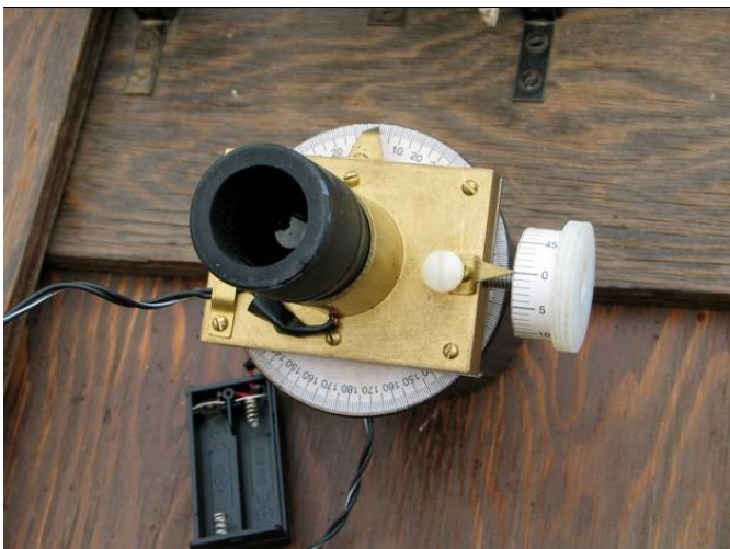
Figure 5: The Filer micrometer the author made for the Hevelius to measure double stars.
