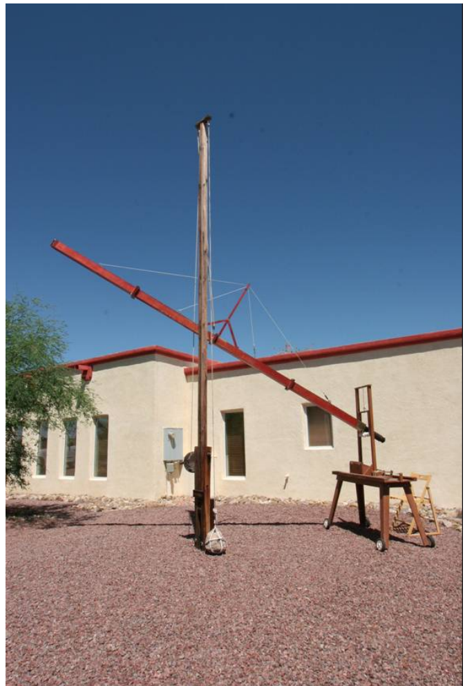
Figure 3: The "Hevelius", the author's 17-foot, long-focal, non-achromatic refractor and its mounting.
