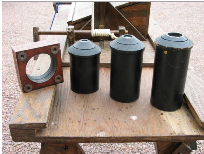
Figure 2: The 2.8 inch, clear aperture lens of the Hevelius and the 150x, 100x and 50x Huygens eyepieces of the Hevelius.
