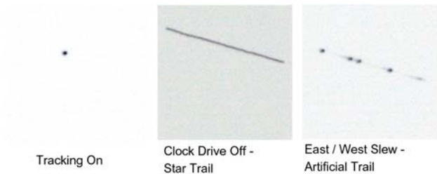
Figure 1: Shows the resulting star trails: clock drive on, clock drive off, slew
