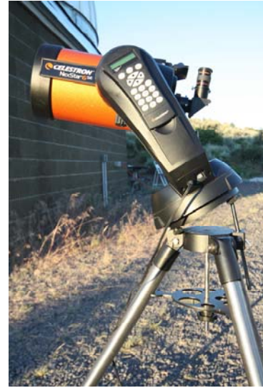
Figure 2: The Celestron NexStar 6 SE mounted on a light tripod for easy portability with an integrated equatorial wedge.
