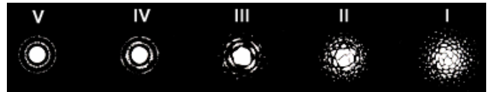
Figure 8: The Danjon scale for atmospheric turbulence.
