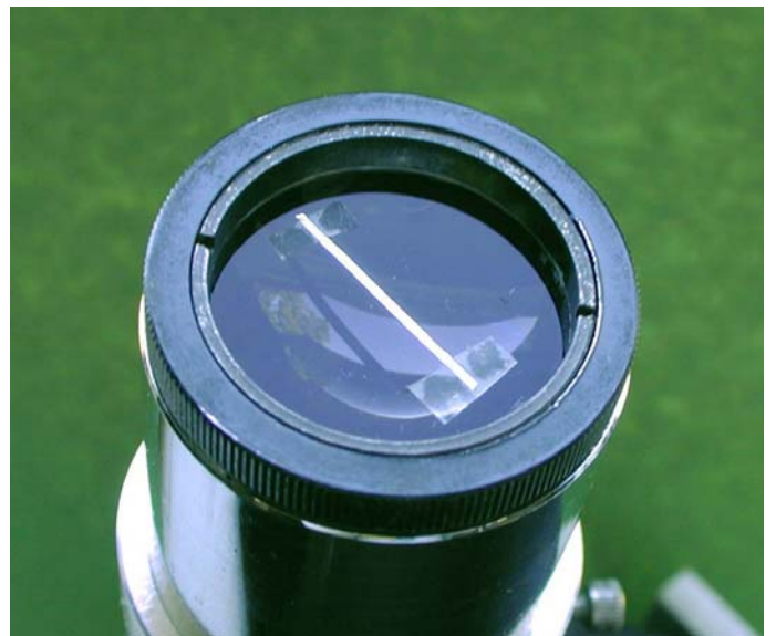
Figure 3: Closeup of Occulting Strip Taped to Field Lens.
