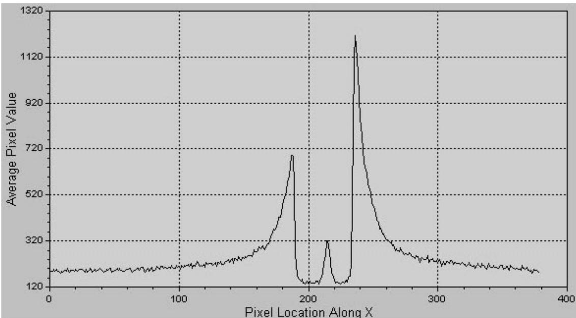
**Figure 1:** This graph shows a line intensity scan perpendicular to the occulting strip and through the occulted image of Spica. The sharp, highly attenuated image of the primary is clearly seen thus permitting accurate centroid determination. Scattered light outside the occulter tapers away to near sky background levels. Figure 5 shows the CCD image used for the scan and includes additional details.
