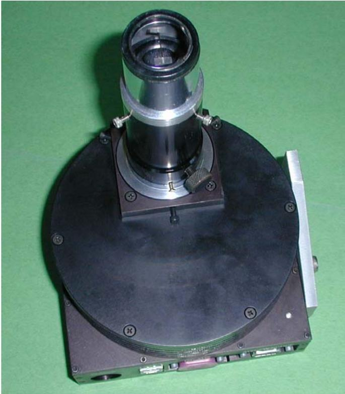
Figure 4: Coronagraph Attached to ST-7 CCD.
