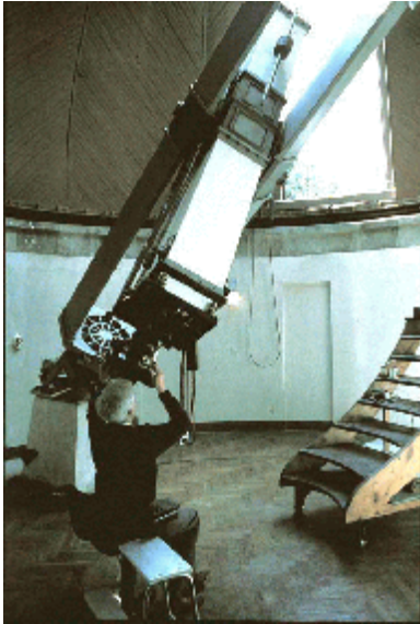
Figure 2: The Vatican's Carte du Ciel astrograph used for zone 2 of the Astrographic Catalog. Photo courtesy Vatican Observatory web site.
