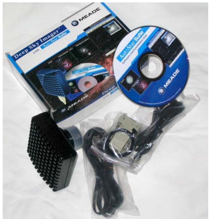
Figure 5: The Meade Deep Sky Imager with heat sink at the camera's rear.
