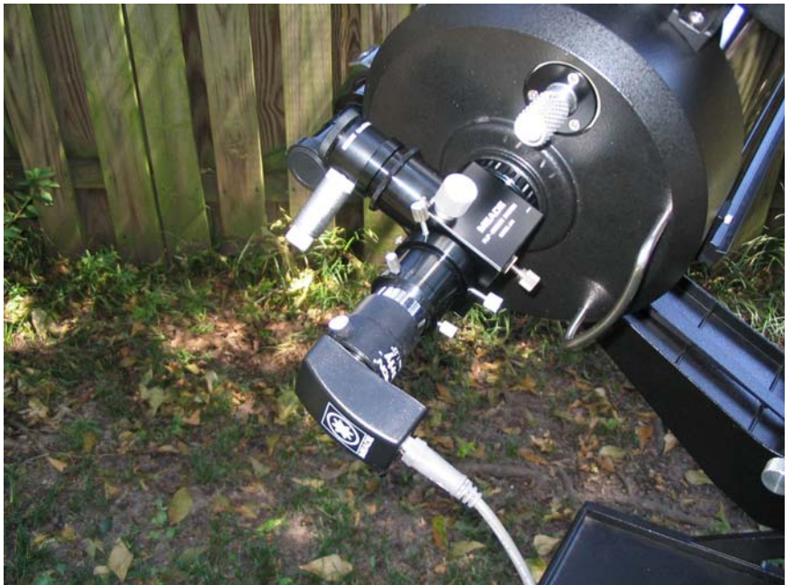
Figure 2: The LPI attached to an alt-az mounted SCT with a flip mirror.
