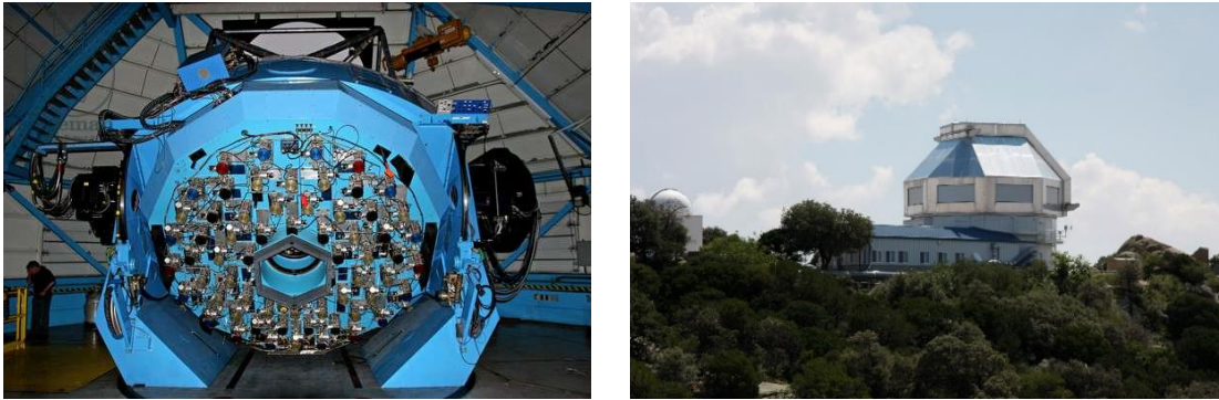
Figure 8: The rear of the WYIN telescopes is covered with actuators that shape the mirror. The octagon-shaped dome is small for a telescope this size thanks to the alt-az mount and short-focus primary mirror.
