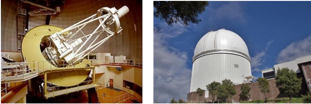
Figure 6: The 3.9-meter Anglo-Australian telescope at the Siding Spring in Australia. It was one of the last large telescopes with an equatorial mount. Later large telescopes utilized alt-az mounts as they are much more compact.
