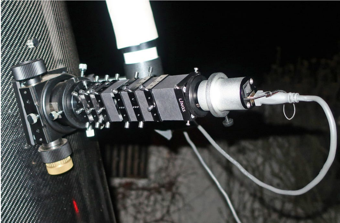
Figure 2 shows the HCDSF instrument first time on telescope in December 2022. In this version tubes of aluminum were used. Mounting plates are still fixed with thumbscrews
