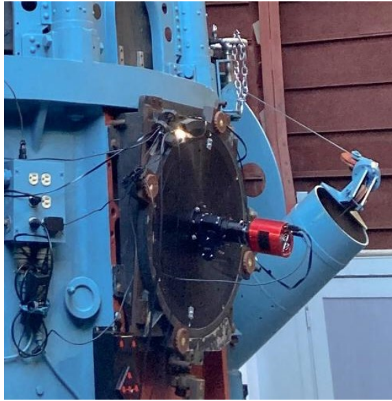
Figure 1. The ZWO ASI 6200MM CMOS camera mounted on the MWO 60-inch telescope.
