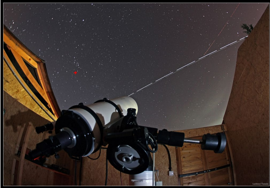
Figure 2: The 250mm Cassegrain reflector of the Castor Observatory, which I use for double star measurements. The image shows the International Space Station and the Space Shuttle Discovery passing overhead on March 23, 2009. (5) Directly above the telescope is the Perseus constellation, in which I marked the location of the Celestial Y with a red cross.
