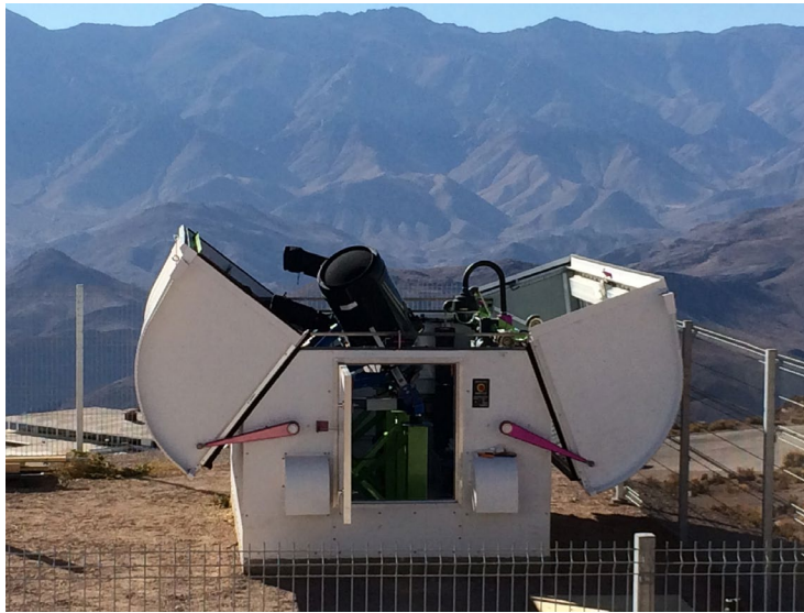
Figure 1. An LCOGT 0.4-meter SBIG robotic telescope in Chile. Image taken by Las Cumbres Observatory.
