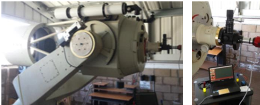
Figure 1: The Orange County Astronomers (OCA) Kuhn 22-inch telescope equipped with a manual flip mirror with an illuminated reticle eyepiece, ZWO motorized filter wheel with standard SDSS filters, a 1.5x Barlow, and a ZWO ASI 290 CMOS camera.
