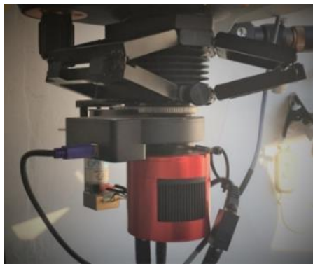
Figure 2: The Fairborn Institute Robotic Observatory (FIRO) 11-inch telescope is equipped with a 1.5x Barlow, motorized ZWO filter wheel with standard SDSS filters, and a ZWO ASI 1600 CMOS camera. It is operated remotely in real time over the Internet using SiTechZWOCam for telescope, focuser, filter wheel and high-speed camera control.
