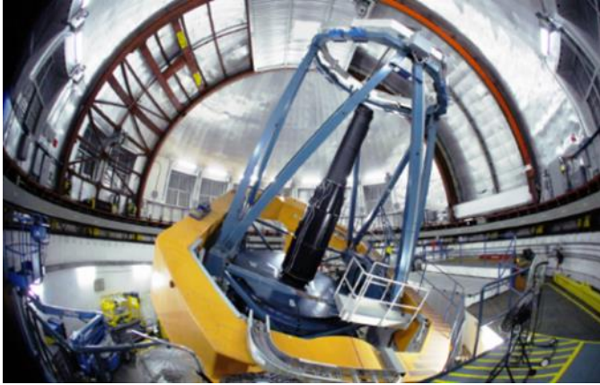
Image 1: The UKIRT telescope with the WFCAM camera. Source: https://news.arizona.edu/story/hawaiian-eye-to-the-sky-now-under-ua-directorship
