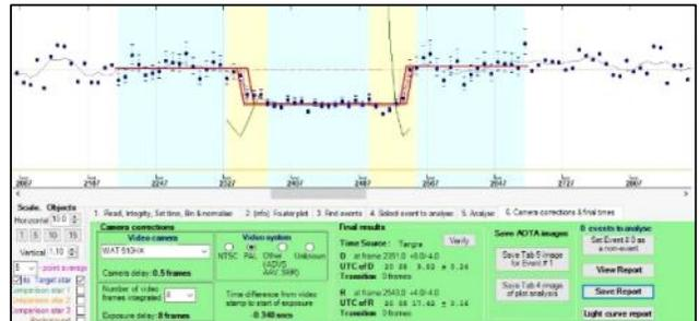
Figure 4: AOTA analysis of occultation 1 with Occult 4<sup>(3)</sup>.
