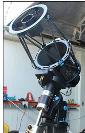
Figure 3. T32 17" PlaneWave f/6.8 CDK Astrograph with FLI Proline 16803 CCD in Siding Springs, Australia.
