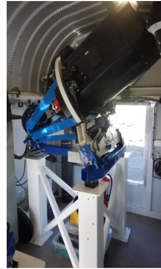
Figure 2: Robotically controlled 0.4m Meade telescope at Siding Springs Observatory, NSW, Australia, with SBIG STX6303 CCD camera.
