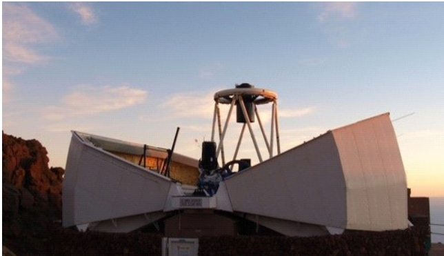
Figure 2. Main telescope structure with a 2-meter and 0.4-meter telescope, Las Cumbres Observatory, Haleakalā Hawaii.
