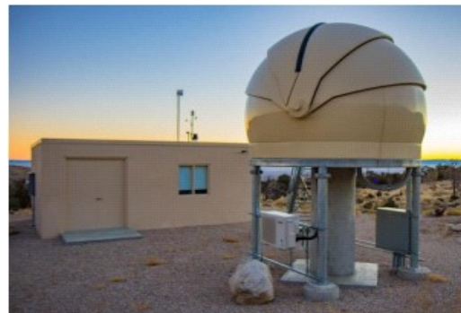
Figure 1. The telescope control software uses the weather station (visible on top of the control room) to determine whether or not it is safe to open the dome. The dome and control room were both painted to match the desert landscape and not detract from the appearance of the park.
