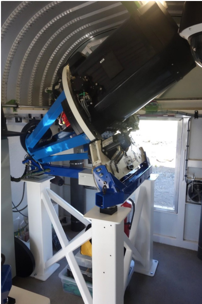
Figure 2. An example model of the 0.4 meter telescope used, built at LCO headquarters in Santa Barbara, California.
