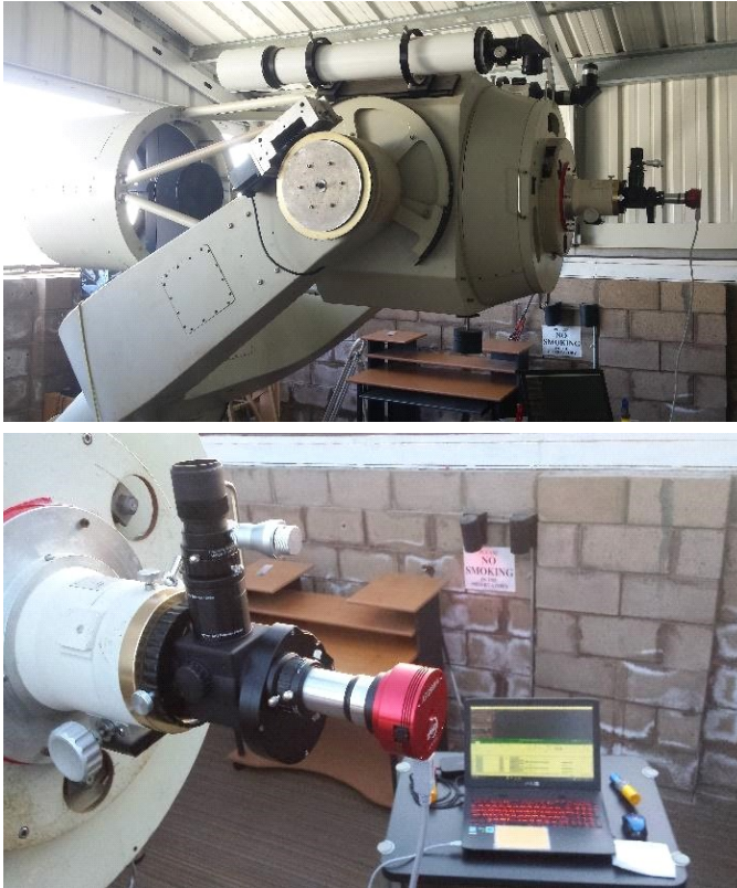
Figure 2. The OCA Kuhn 22-inch Cassegrain telescope instrumented for Speckle Interferometry. Camera, power, control and image acquisition are through the single blue USB3.0 cable to the laptop computer at lower right, running FireCapture software.
