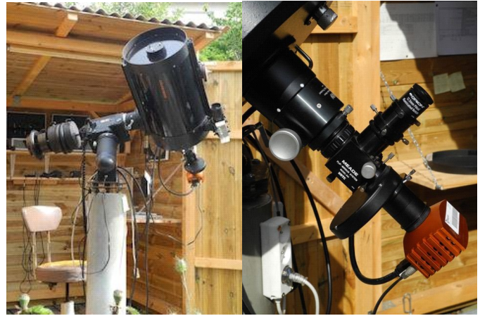
Figure 3. – Instrumental setup in Clermont-Ferrand. Left : C11 on equatorial mount. Right : optical train (flip mirror, centering eyepiece, filter wheel, projecting eyepiece and ADC – inside the tube between the filter wheel and the camera – and Raptor Kite EM-CCD
