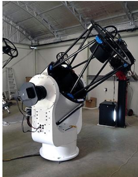
Figure 1. Planewave 27" (0.7m) CDK700WF. CDK Astrogaph with TEL 0.70-m f/6.6 reflector and CCD in Siding Spring, Australia
