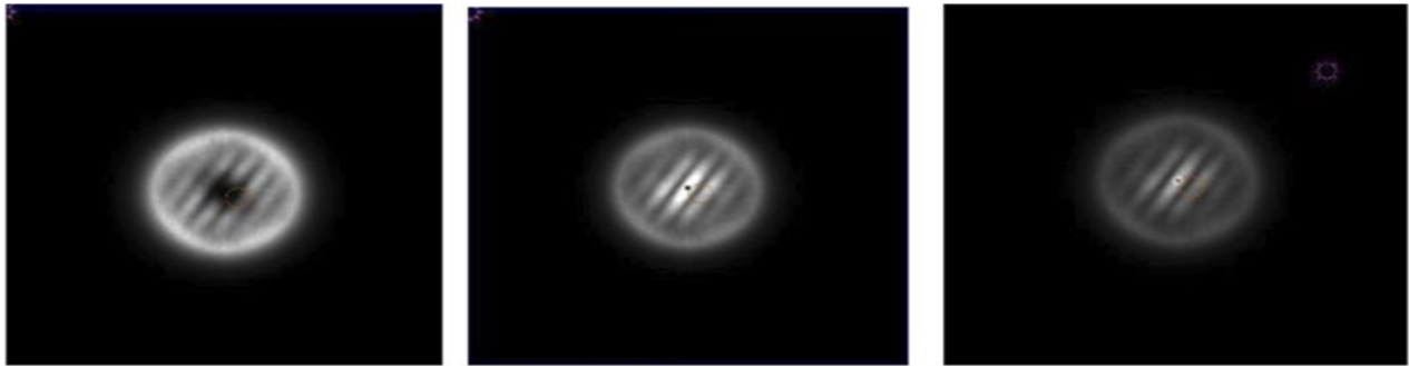
Figure 6. Gaussian high pass filter examples. Left - too wide (cuts off the central peak and the fringe pattern), centre - set correctly, right - too narrow (allows the central peak to be seen). Image adapted from Harsahw et al. (2017)
