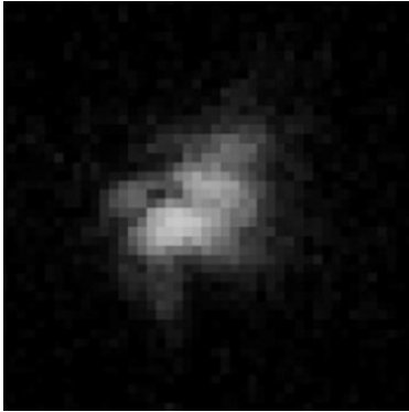
Figure 5. 0.004 second exposure of a reference star (Fomalhaut) with 0.2m telescope
