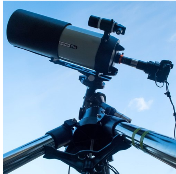
Figure 2. Celestron Edge HD 800 with Canon 6D on Losmandy G11 mount
