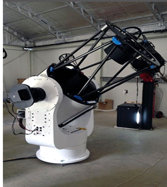
Figure 2. T27 - Planewave CDK 0.70 m Reflector Telescope. ( http://www.itelescope.net/telescope-t27/ )
