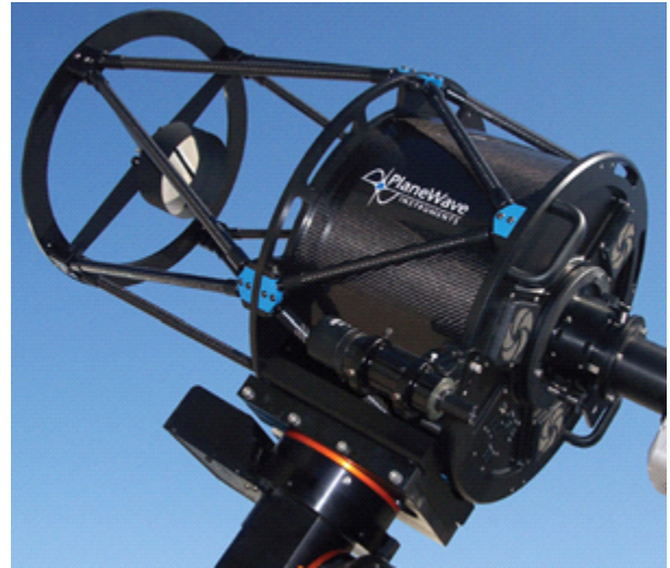
Figure 4: The PlaneWave Instruments CDK17 astrograph telescope similar to the telescope used for observations at SRO.
