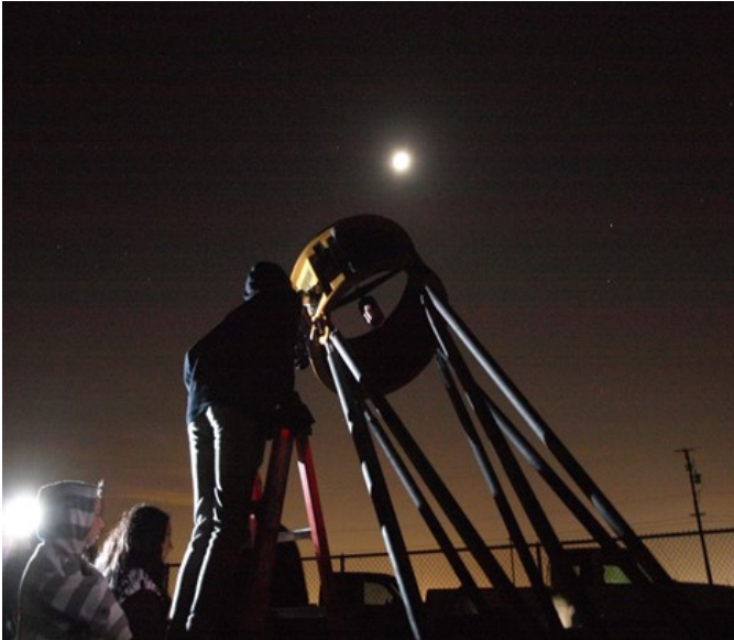
Figure 2: An image of the 22-inch Newtonian Alt/ Az telescope with a Celestron 12.5 mm Micro Guide eyepiece.
