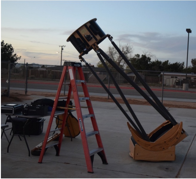
Figure 2: This is a picture of the telescope used to collect digital data of the double star. Picture taken by Chris Estrada.
