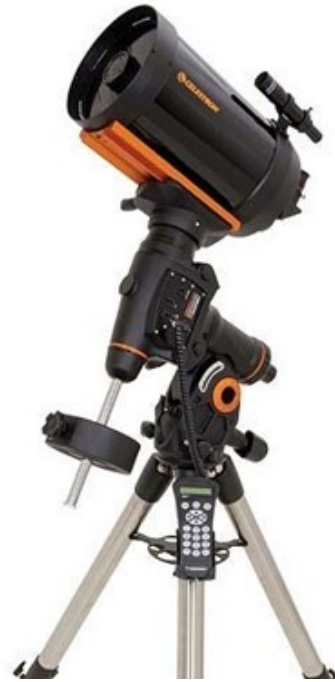
Figure 2. The telescope used by the observers - Celestron C8 Schmidt-Cassegrain with Advanced VX Mount
