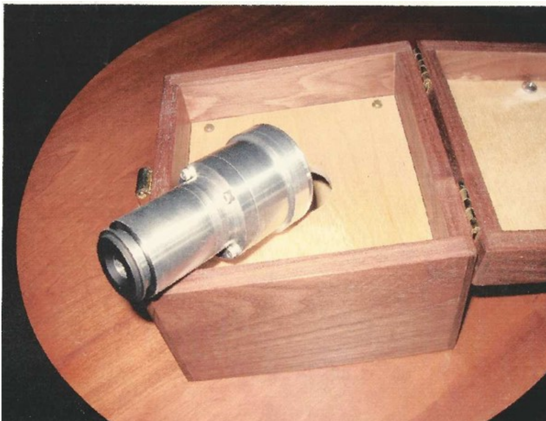
Figure 1. A photo of LSO's new stellar coronagraph. A Lyot stop is incorporated and is easily accessed by removing the screws seen near the barrel's mid-point. The telescope is focused on the field lens/occulting mask seen at the left. The CCD bolt-up flange is to the far right.
