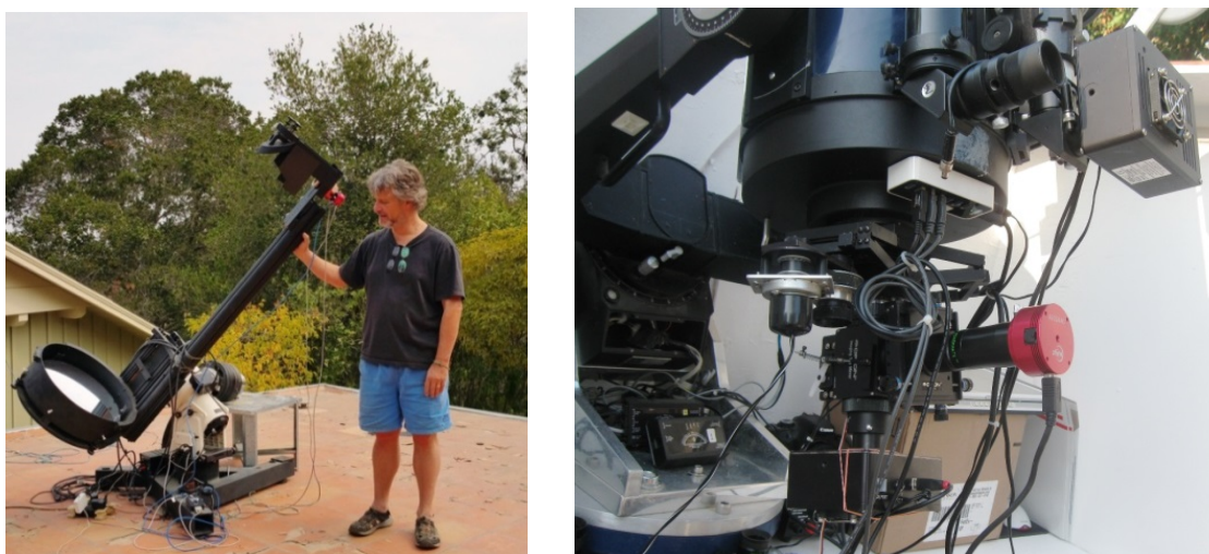
Figure 5. Left: Benoit Shillings, with his 0.5-meter telescope, made the first close double-star speckle interferometry observations with the ZWO ASI 224MC camera. Right: close-up of the instrumentation at Russ Genet's Orion Observatory. The ZWO camera is behind a Tele-Vue 2.5-power Barlow lens.
