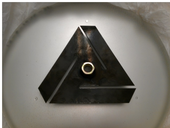
Figure 6. Attached mirror support fixture and sapphire pads
