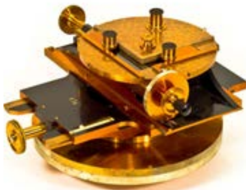
Figure 2. The filar with micrometer used on the 36 inch refractor at the Lick Observatory.
