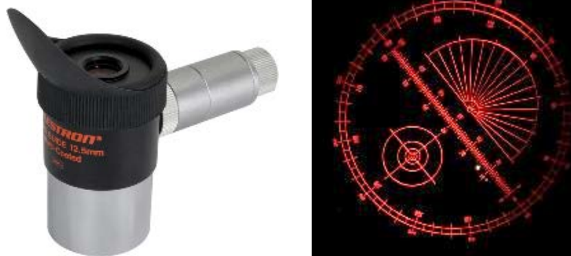
Figure 13. A Celestron astrometric eyepiece, along with a photo of Albireo in the astrometric eyepiece showing a measurement of the separation.
