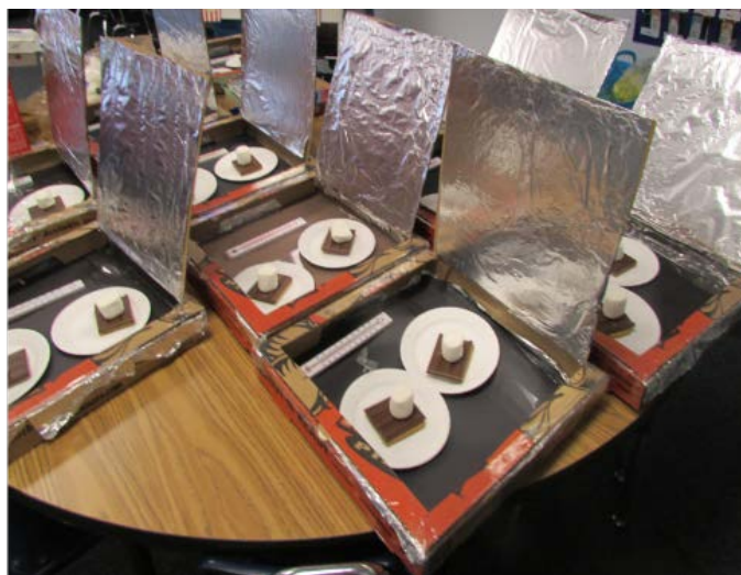
Figure 1. Solar Oven Engineering Activity
