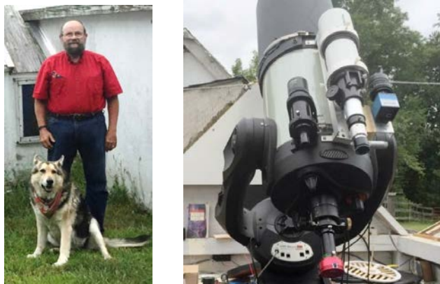
Figure 6. Clif Ashcraft and his Night Assistant, Boomer. Celestron C-11 telescope equipped with the ZWO ASI 224MC camera behind a 3X Barlow lens.
