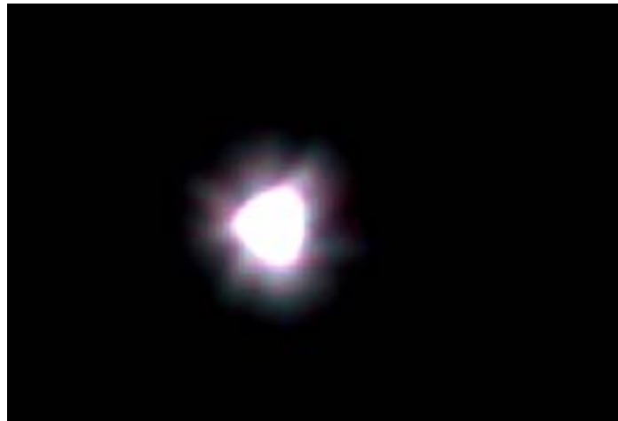
Figure 13. Webcam capture for alignment mirrors using white LED
