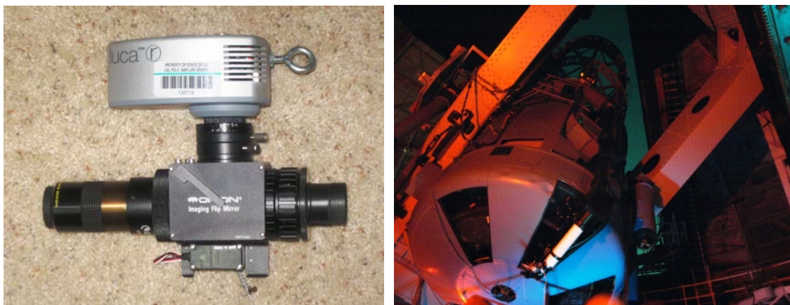
Figure 2. Left: close-up of the speckle camera for the 100-inch checkout with its Andor EMCCD camera, Orion flip mirror, and eyepiece. Light from the telescope entered from the right. Right: the camera installed on the 100-inch telescope at the end of the white optical extension.
