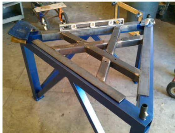
Figure 3. Mirror support frame being fitted to telescope base
