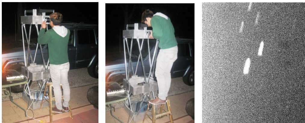
Figure 8. Installment of CCD camera, left, and image of drift captured, right.
