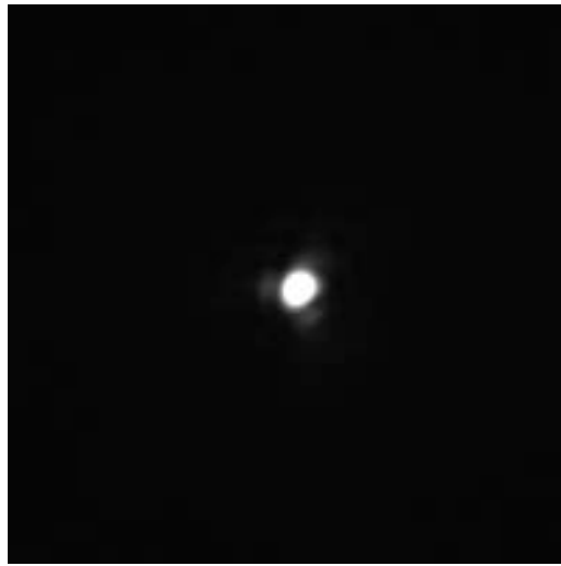
Figure 14. QHY capture for aligned mirrors using green LED
