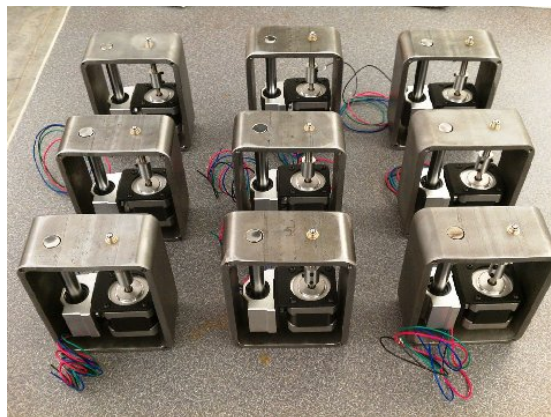
Figure 4. Active optics actuators before attaching side covers
