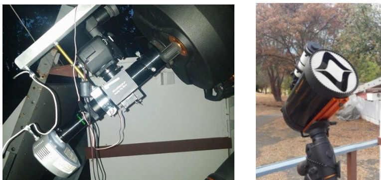
Figure 6. The left image shows the back end imaging components, the right image shows the Gaussian Donut mask on the C-11 telescope.
