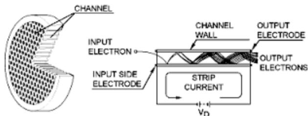
Figure 3. A Microchannel Plate, left, along with an individual microchannel, right.
