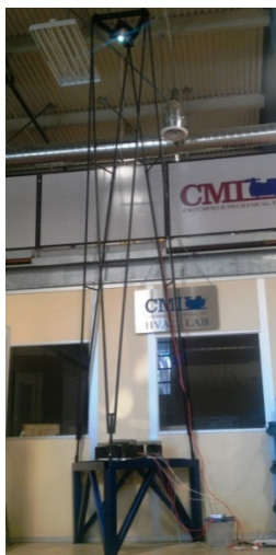
Figure 5. The three mirrors on their positioners with the control electronics and the vertical test stand.
