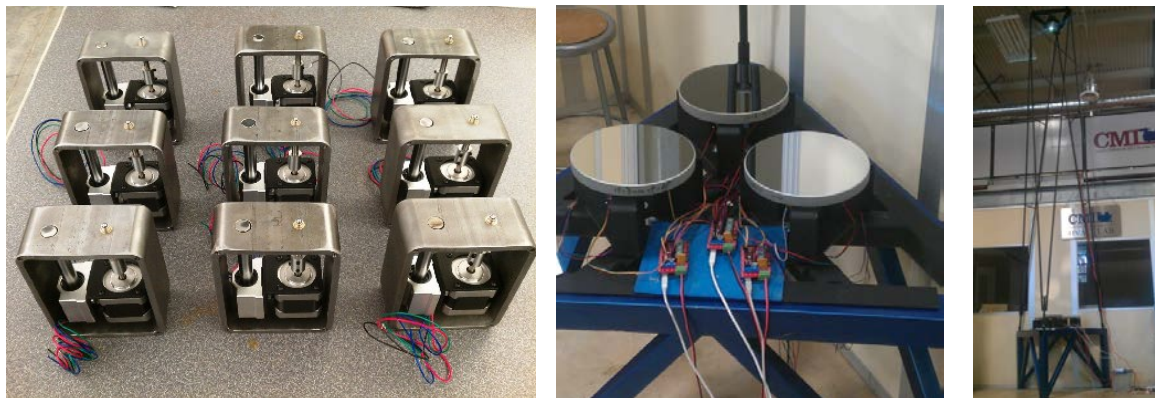
Matthew Clause, a mechanical engineering graduate student, designed and built the nine high-precision actuators on the left that supported three spherical mirrors, center, all mounted in a test tower, right, with a high brightness LED and astronomical camera at the center of curvature to enable optical alignment through the use of interferometry.
