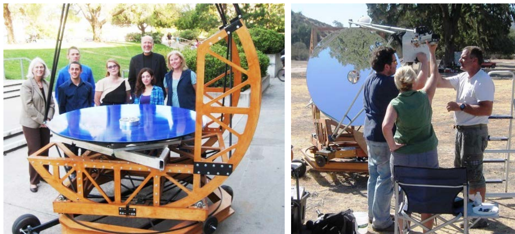
Left: The Cal Poly 1.5-meter experimental light-bucket flux collector telescope (the blue coating on the mirror protected the mirror during assembly). Right: installation of ultra-high-speed photometer for intensity interferometry field tests.
