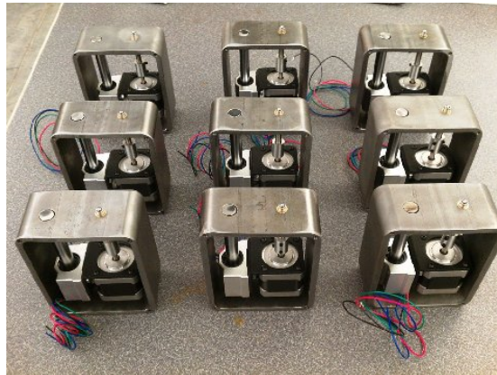
Figure 4. Active optics actuators before attaching side covers
