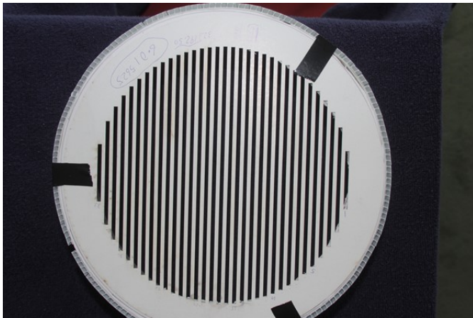
Figure 1. Photograph of the mask with 6 mm slit spacing.
