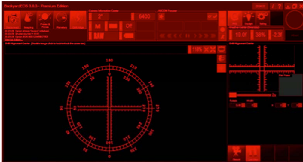
Figure 3: Screen capture image showing the protractor and linear reticule scales for performing drift alignment in BackyardEOS, here used to make separation and PA measurements. Note that only one half of the linear scale was used since the width of the center division is variable.
