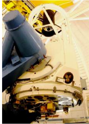
Figure 2. The 2.1-m f/7.6 telescope at Kitt Peak National Observatory dwarfs our portable speckle camera.
