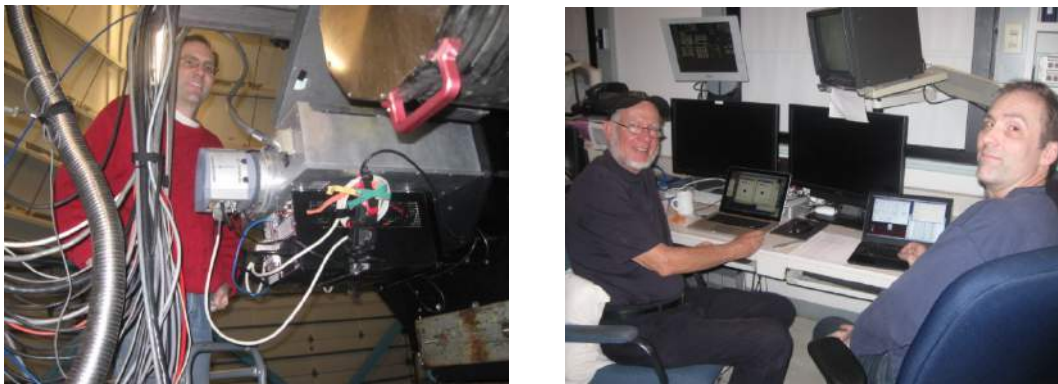
Figure 11. Elliott Horch and his speckle camera on the 3.5-meter WIYN telescope. One of the Andor EMCCD cameras can be seen. The other is out of view on the other side. The black PC can be seen fastened to the bottom of the system (left). Russ Genet operates the two cameras from the warm room while Elliott operates the log (right).
