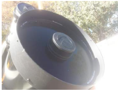
Figure 24. The aperture of the Celestron C11 Schmidt–Cassegrain telescope. Note how the secondary mirror embedded in the corrector plate obstructs the aperture.
