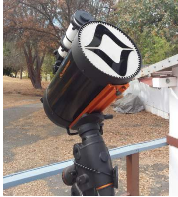
Figure 29. The double Gaussian mask applied to the Celestron C11 telescope. The mask's outer gear teeth are designed to interface with an automatic rotation mechanism (not pictured).
