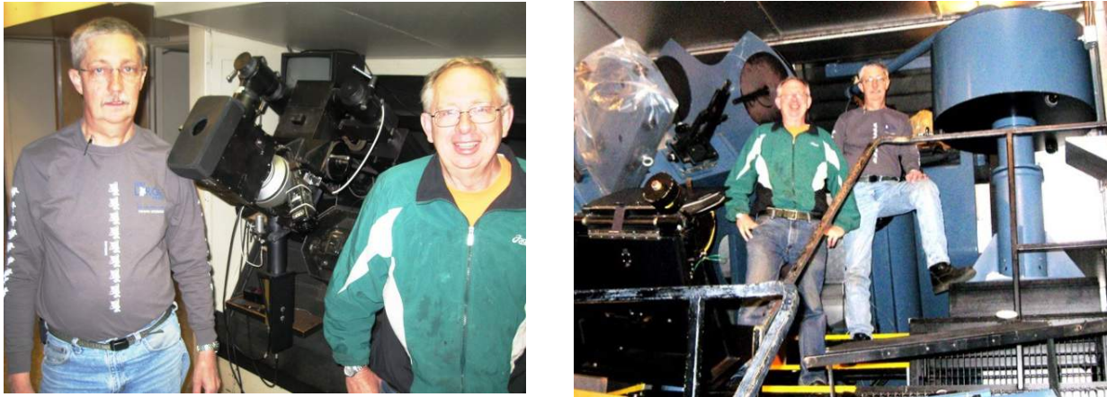
Figure 20. Wayne Green and John Kenney at the top, slit end of the spectrograph (left). The light from the slit then enters the basement room which contains several spectrographs including a high resolution Echelle (right).
