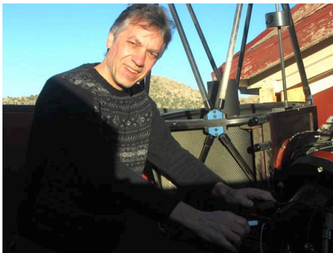
Dan installing high-resolution on-axis encoders on the Pinto Valley Observatory's telescope mount. In the end it took hand files and Scotch tape to get them to work.
