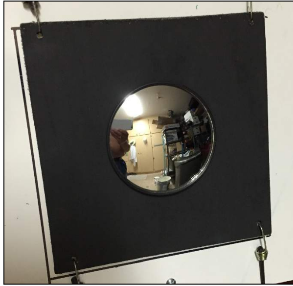
Figure 6. The convex mirror target for the laser tests.
