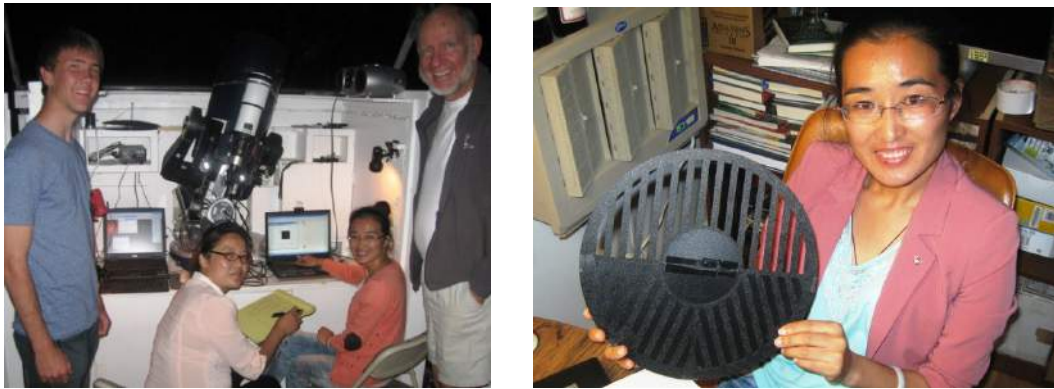
Figure 10. Eric Weise, Chaoyan Wang, Yuanyuan Ding, and Russ Genet (left). They made speckle interferometry observations of double stars with the 0.25-meter telescope at the Orion Observatory. The slit mask used for pixel scale calibration (right).
