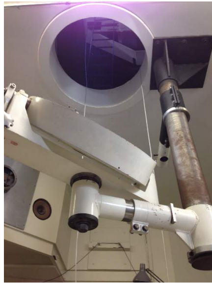
Figure 2. The East Auxiliary light feed port in the observation room ceiling We ended up with the optical shown in Figure 3.
