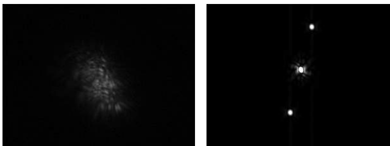
Figure 5. Raw speckle image of a double star (Wiley 2014) and the processed autocorellogram using Plate Solve 3.
