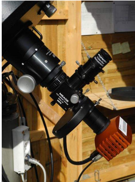
Figure 2. Optical train for measurements. From left to right: focuser (Crayford), flip-mirror (with crosshair eyepiece), filter wheel, Powermate, Raptor Kite EM-CCD (with power supply and CameraLink cables). The ADC is not present here. It is normally mounted just before the Powermate.
