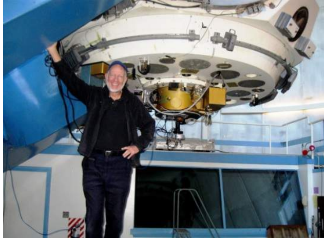
Figure 3. The Cassegrain focus of the 2.1-meter telescope. To the right of Genet is the gold-colored acquisition-guider unit. Below the acquisition-guider is the black-colored Barlow lens, filter wheel, and silver-colored Andor EMCCD camera of our portable speckle interferometry system.
