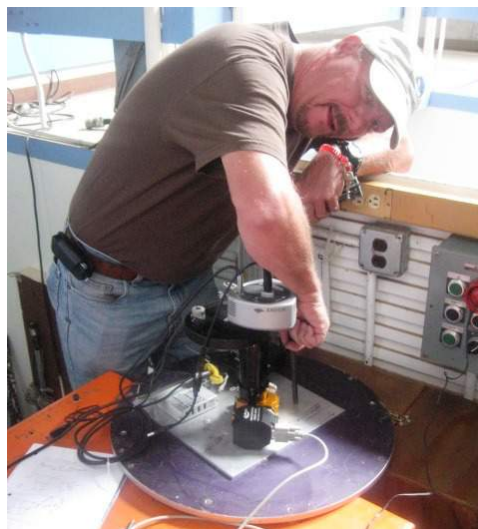
Figure 6. Thomas Smith attaching speckle camera to the Kitt Peak-provided plate.
