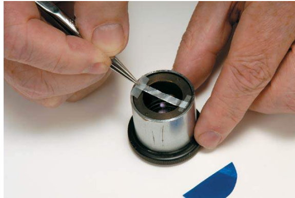
Figure 3. Aluminum foil occulting bar applied to an eyepiece (Sinnott & Ashford 2005).
