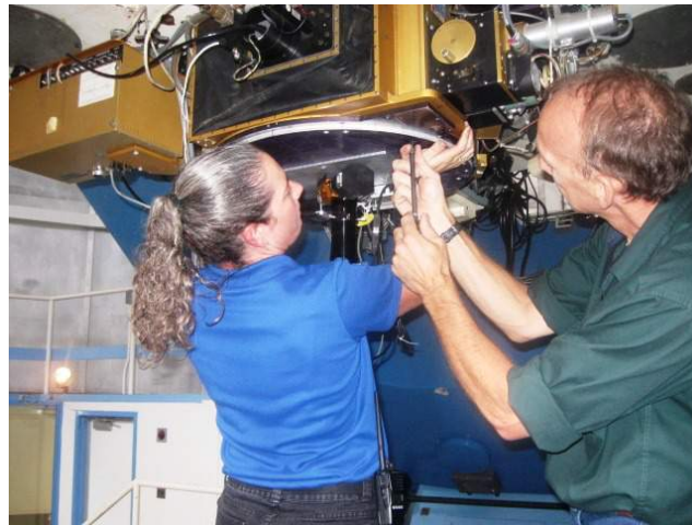
Figure 7. Installing the camera assembly on the telescope.
