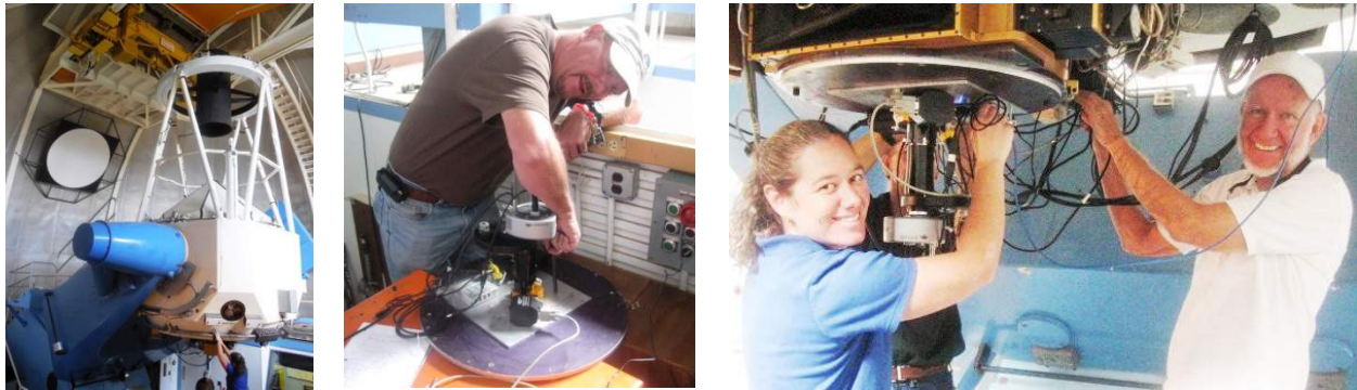
Figure 14. Mathis installed counterweights (left), Smith fastened the EMCCD camera to the interface plate (center), and Mathis and Genet fastened down the cables (right).
