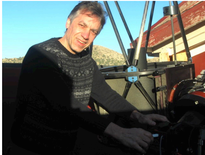
Dan installing high-resolution on-axis encoders on the Pinto Valley Observatory's telescope mount. In the end it took hand files and Scotch tape to get them to work.
