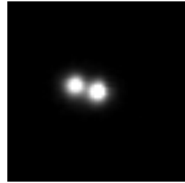
Figure 2. Epsilon Lyrae south-east pair, STF2383CD. REDUC Shift & Add image of best 42 (8%) of 495 frames from drift "a."
