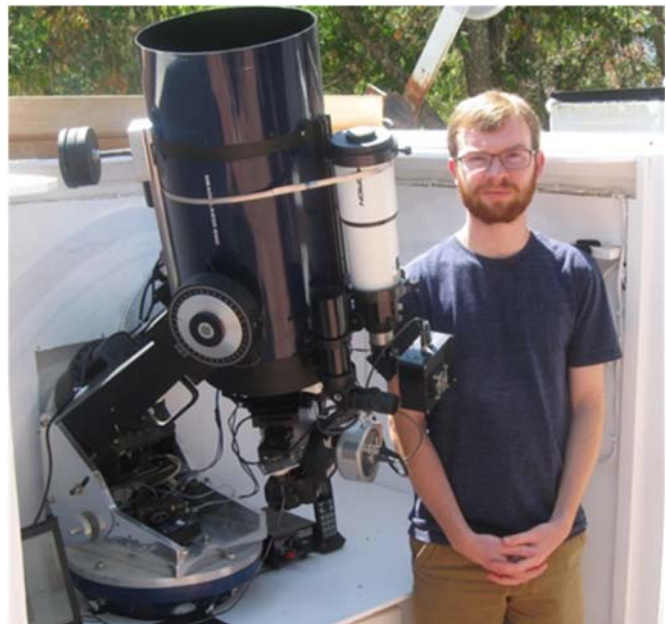
Figure 3. Alex Teiche stands beside the Meade/Sidereal Technology 0.25-meter Schmidt-Cassegrain telescope at the Orion Observatory near Santa Margarita Lake, California. This photo was taken the morning after first automation was achieved.
