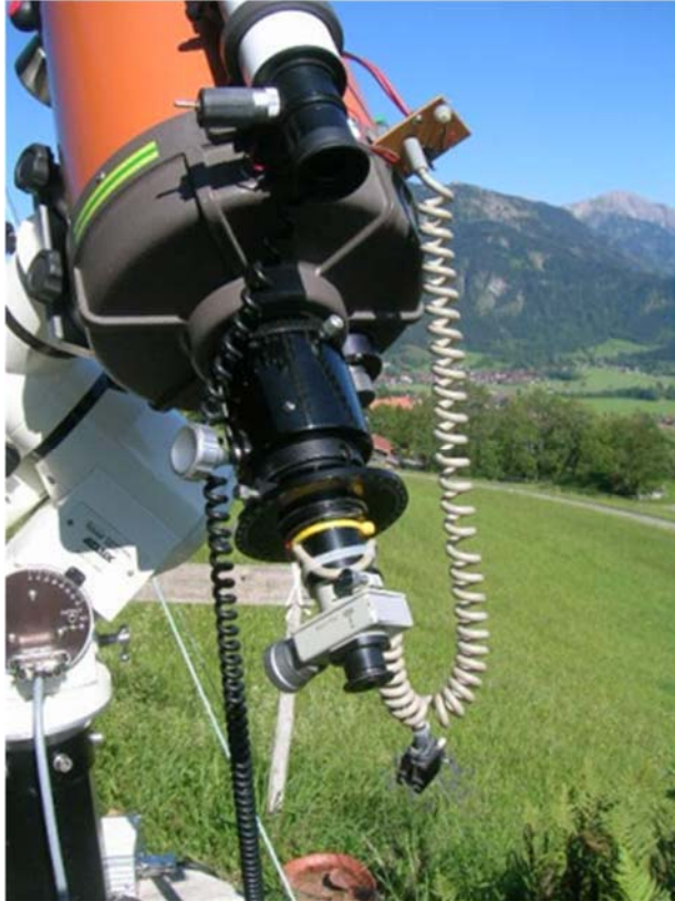
Figure 1. Orange C8 used in this study. The attached micrometer and PA circle are also visible just above the eyepiece.
