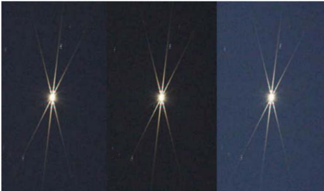
Figure 3. Bahtinov diffraction images. The central image shows the proper orientation of the central spike to attain maximum focus. (Wikipedia, http://en.wikipedia.org/wiki/Bahtinov_mask .)
