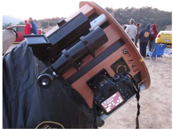
Figure 3: Obsession alt-az telescope with Canon T2i DSLR at prime focus
